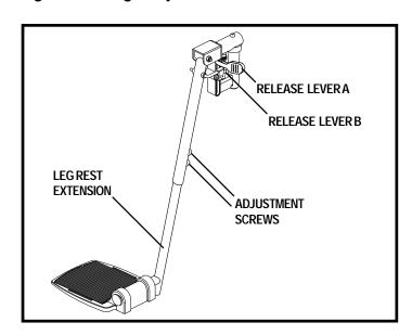
Figure 21. Elevating Leg Rests
